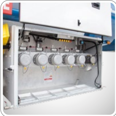
PUMP FORCED DISCHARGE THROUGH 4" API ADAPTERS
